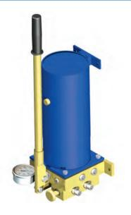
Hand pump operates in combination with double acting cylinder. High-pressure hose of 3 m length is included in delivery. Cylinder has to be ordered separately. Robust design, high precisely part treatment, high quality seals provide long time exploitation of the hand pump. Delivered pump is filled with oil and ready for use. Before use release the breather screw and retight the unloading handle.
